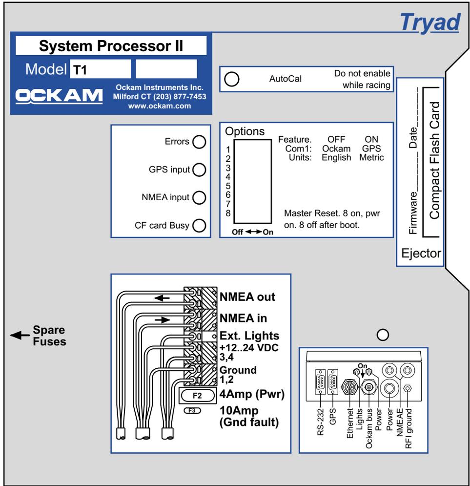
The Tryad T1 CPU is the brain of the Ockam system. It gathers information from various interface components, controllers and serial ports, calculates outputs, and sends data to displays and other data targets. The CPU also includes a clock and calendar which provides various timing functions to the system.
