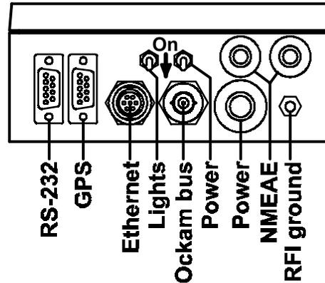
Setting option switch #1 at power up will temporarily set the RS-232 port to 4800,N,8,1, and source GPS data. In other words, RS-232 would look like a GPS.
