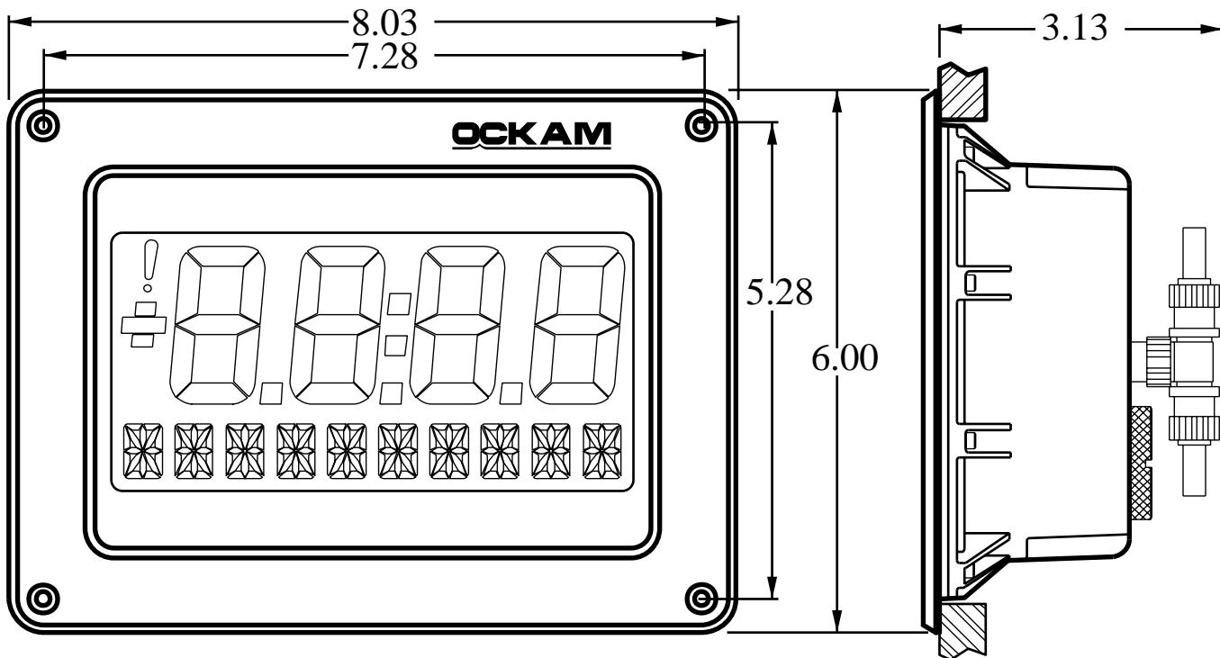
**Large Format Remote Display** is usually used in locations where it is inconvenient to use cards to change the displayed function, like on a mast pod. The large format makes it ideal for mounting where it will be viewed from a long distance away.
